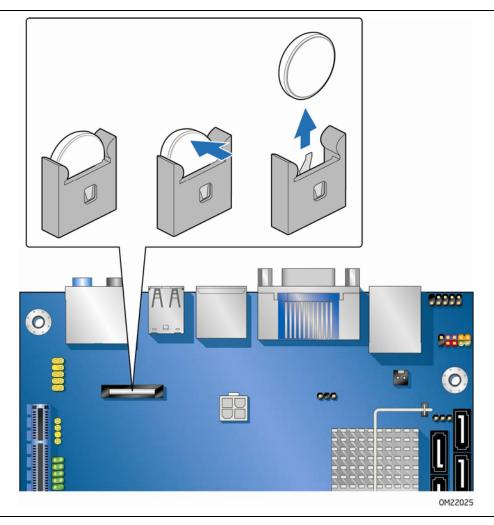
Figure 25. Removing the Battery
